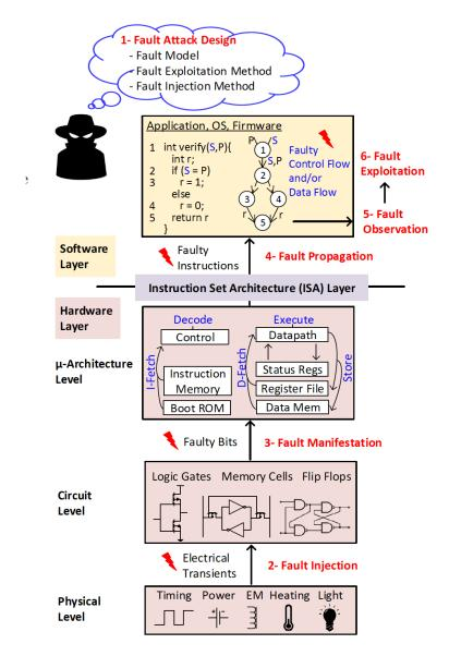
Figure from "Fault Attacks on Secure Embedded Software: Threats, Design and Evaluation", *Bilgiday Yuce, Patrick Schaumont, Marc Witteman*
